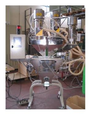
The mixer consists in the basic model from supply hoppers for four components and a below placed balance where the compounding is done. One of the components is given to the balance, the other up to four components added from dosing units with valves or, for high output rates, with screws in high precision. The mixed material is then dropped into a supply bin, where an intake tube may be connected directly.
