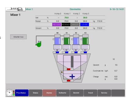
Dosing throughput depends on density and granularity of used material.
