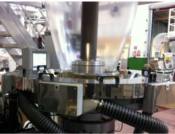
For a better analysis of the film production process, combine the film thickness measurement and control system with our webMIP film production management system.
