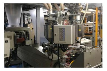
The weighing and dosing station **GDS** is designed for mono- and co-extruders working with granule resin at up to 500 kg/h throughput (**GDS**) or above (**GDS/S**) and to integrate – measure and control - up to four or six blend, additive or master batch components. All hoppers made of stainless steel with particularly effective material supply.
