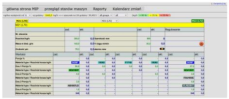
The product quality, e.g. at film production plants, can be improved by analyzing production's quality parameters as film weight, thickness, thickness profile and compliance with the recipe over any time period (shift, month, order), in case of a customer's question.
