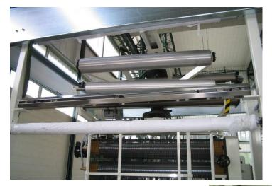
A flat-lying film tube is guided over the measuring frame. Infrared sensors move perpendicular to the film edge on both sides of the measuring frame. As soon as a film edge is detected, the correct width is cyclically calculated. The measurement has no effect on the surface of the film.
